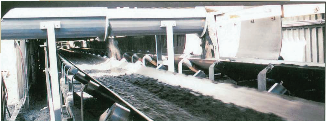
Twin “Live Bottoms” Volumetric Feeders in a Blending Application
